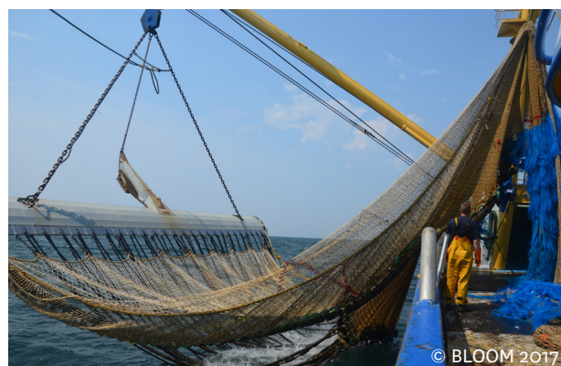
Electric 'pulse' trawls in the North Sea.
